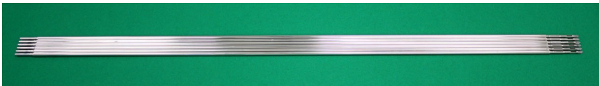
U-Pu-Zr fuel pins fabricated for Irradiation experiment in Joyo
