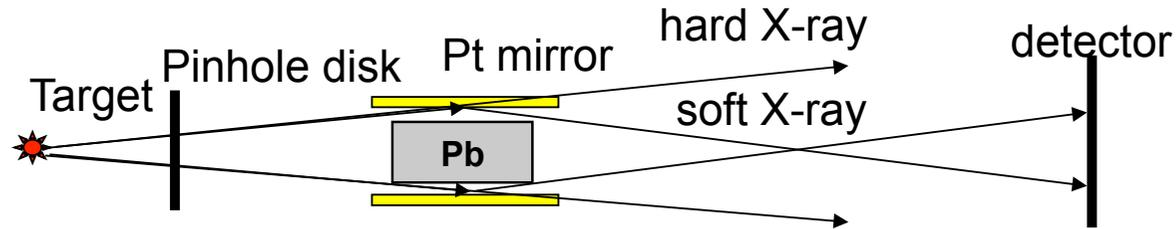
Hard x-ray shielded cathode for x-ray streak tube
