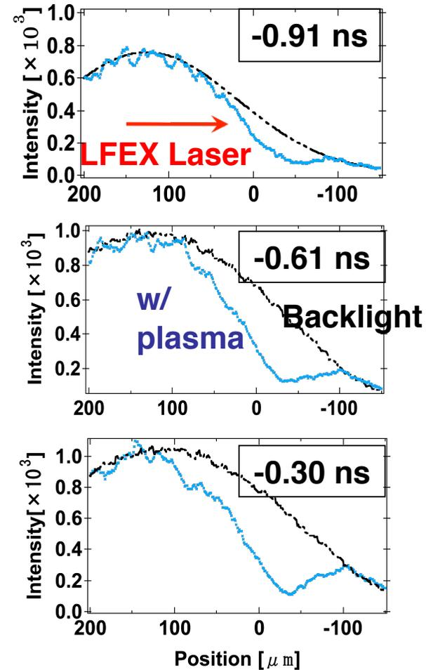
We have to reduce the pre-formed plasma to increase the coupling efficiency of heating.
