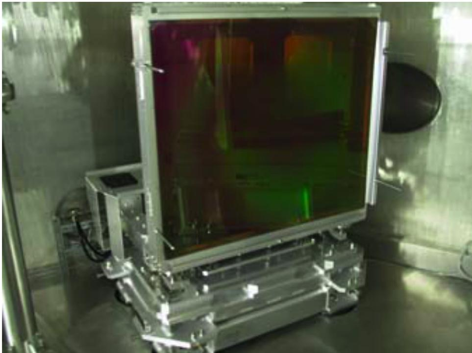
Off-axis parabola mirror installed into chamber
