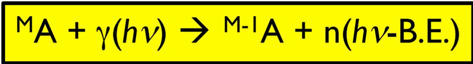
Neutrons in the MeV range can be created due to  $(\gamma, n)$  reactions (*photo disintegration reactions*) in materials in and around the target.
