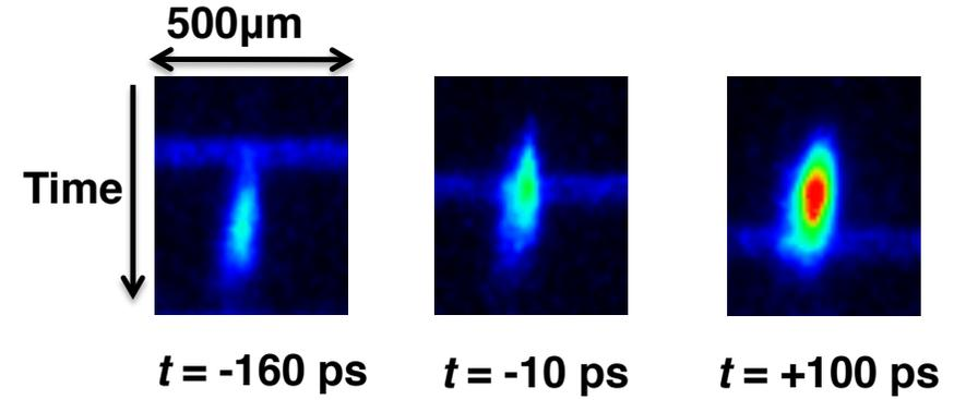
Relation between hard x-ray signal and the imploded core plasma
