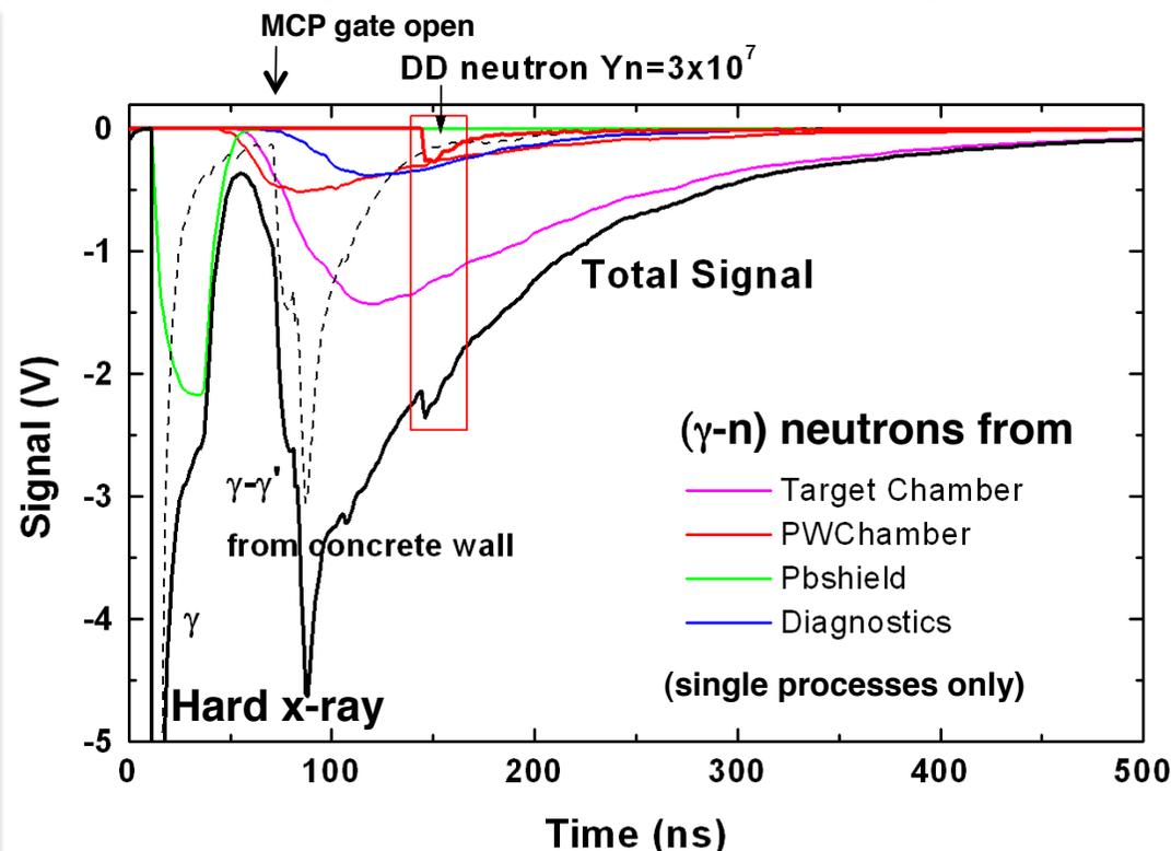
**Now we know nature of the background signals, and can accurately identify the DD neutron signal even with the heavy backgrounds.**
